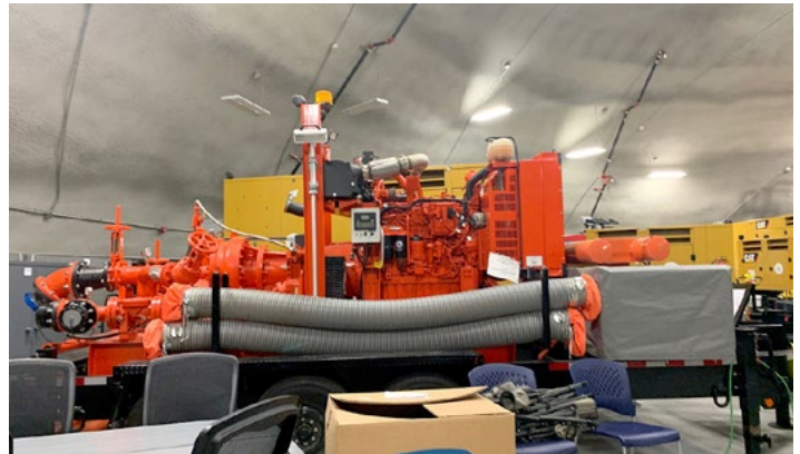
A Godwin pump, used to provide water to key systems, sits in a storage dome where backup equipment is kept at our Surry Power Station in Virginia.
