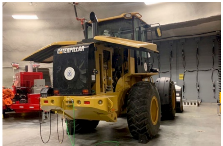
A front loader used to move debris and tow equipment into location, also housed in Surry’s FLEX equipment storage dome.
